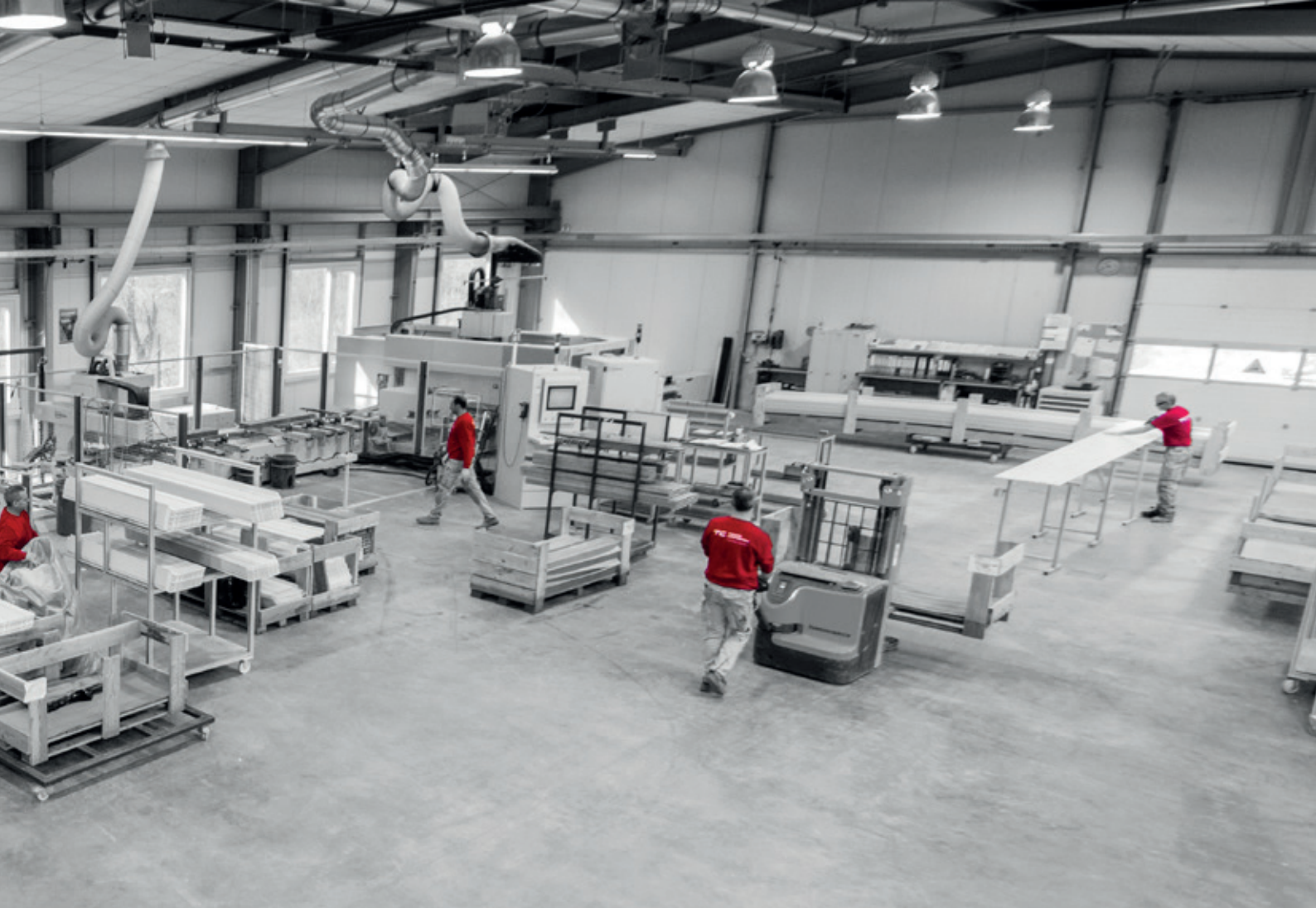
Machine hall of Techno-Composites Domine GmbH in Meppen, Lower Saxony. This is where CNC machining of the GRP profiles takes place.
